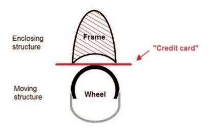
practical way of confirming the existence of fairing on a moving part such as a wheel: it should be possible to pass a rigid card (like a credit card) between the fixed structure and the moving part.
