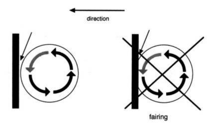
A fairing shall be defined as the use or adaptation of a component of the bicycle in such a fashion that it encloses a moving part of the bicycle such as the wheels or the chainset. Therefore, it should be possible to pass a rigid card (like a credit card) between the fixed structure and the moving part.
