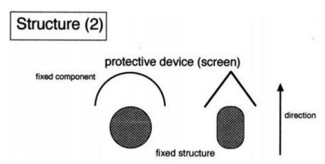
A protective screen shall be defined as a fixed component that serves as a windscreen or windbreak designed to protect another fixed element of the bicycle in order to reduce its wind resistance.
